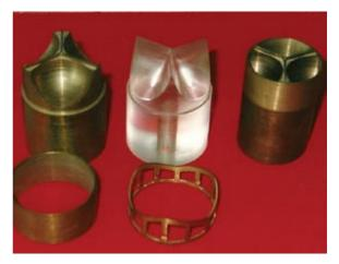
Fig 1. Moulds for building the first experimental pericardial valves
