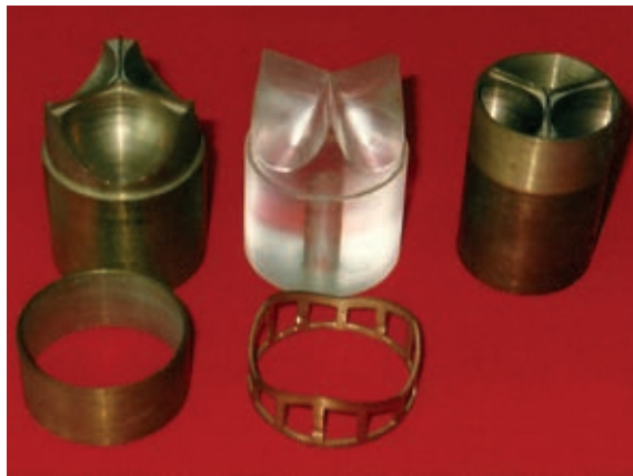
Figure 1: Moulds for building the first experimental pericardial valves.
