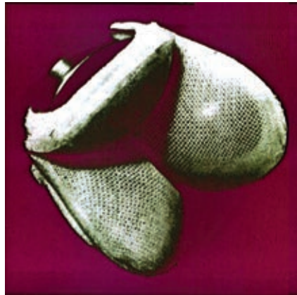
Figure 2: Original photograph of a three cusp valve made of Dacron mesh
