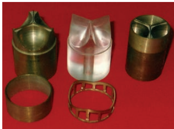
Figure 3: Moulds for Valves.
