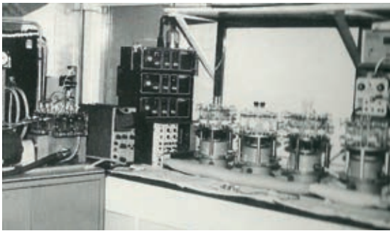
Fig 14: Heart Valve durability testers.
