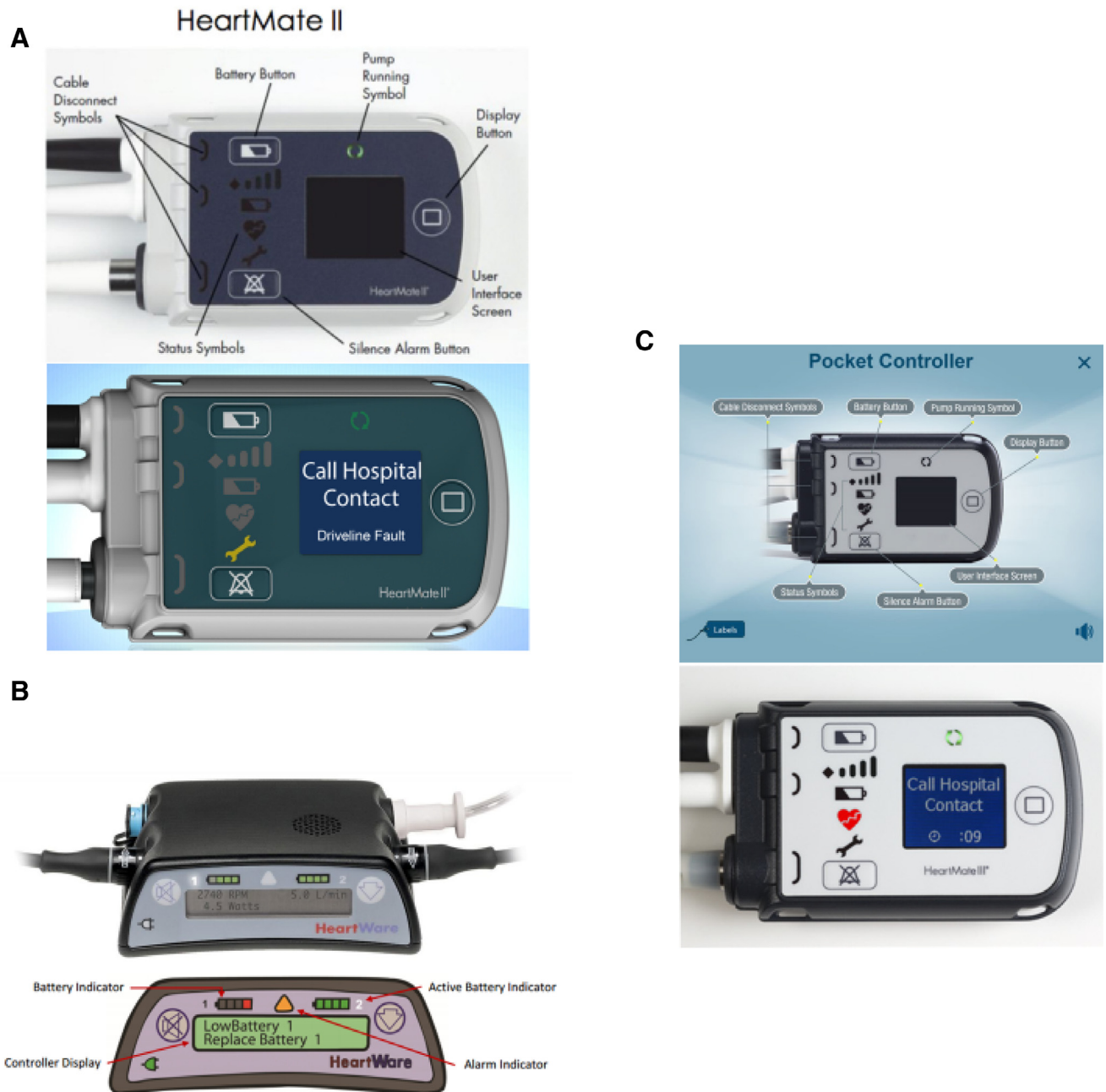
Figure 2 Left ventricular assist device (LVAD) controllers with an alarm display. (A) HeartMate II pocket controller showing controller display/buttons (top) and driveline fault alarm with a yellow wrench (below). The patient is instructed to contact the ventricular assist device (VAD) team for further advice on troubleshooting and management. (B) HeartWare HVAD with controller display/buttons (top) and low battery alarm (below). The patient is instructed to replace the battery. (C) HeartMate 3 pocket controller (top) and red heart alarm (below). The patient is instructed to call the hospital contact (LVAD program).
